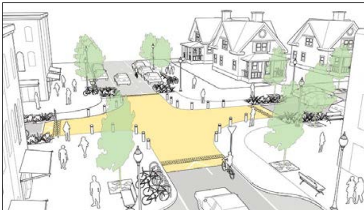
A raised intersection is proposed at the intersection of Main and Morgan. This is a public art opportunity, slows vehicle speeds, increases accessibility, and improves pedestrian safety & usability. (Image: NACTO)
